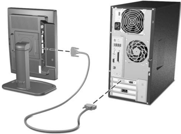
Connecting the DVI-D Signal Cable
