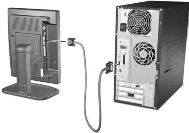
Connecting the VGA Signal Cable
